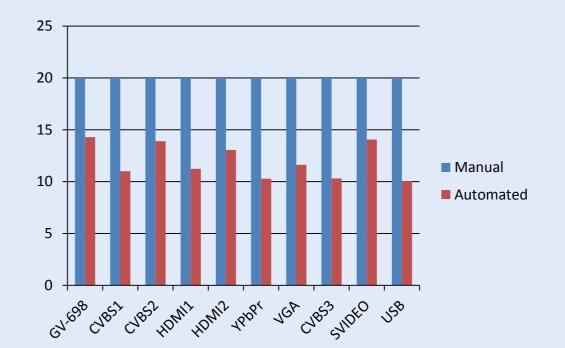
Lessons learned from verification of TV sets: comparison of the times needed by automated and manual verification for several input interfaces
