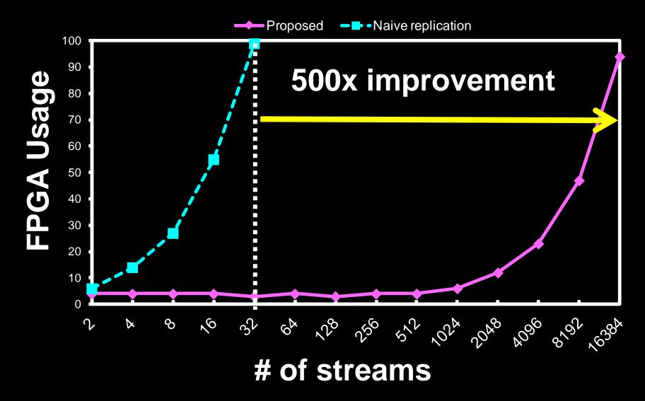
FPGA Usage = max(block mem usage/block mem avail, slice usage/slice avail) \* 100
