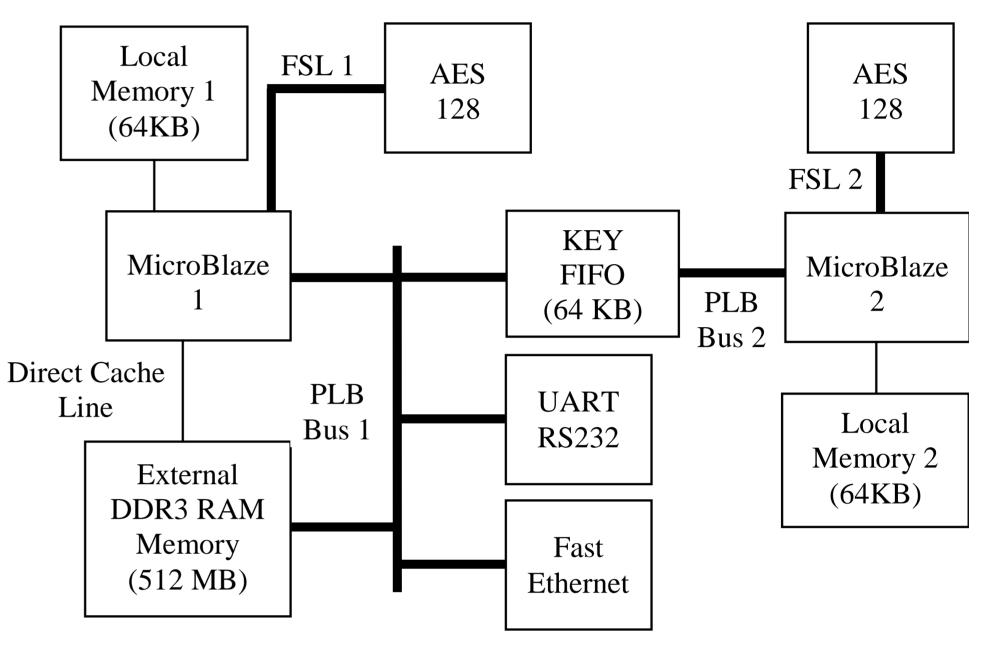
The first MicroBlaze takes care of managing the complete GKM and KSM. The second MicroBlaze takes care of calculating new keys (two encryptions are need for one key) and storing in a Key FIFO. MicroBaze 1 take new keys from this Key FIFO. The next figure shows the AES implementation:
